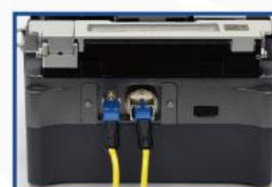
Power Meter & Fault Locator
