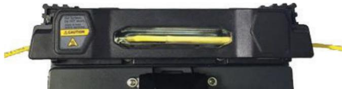
4| Remove the sleeve protected fiber by opening the cover when the cooling is completed.
