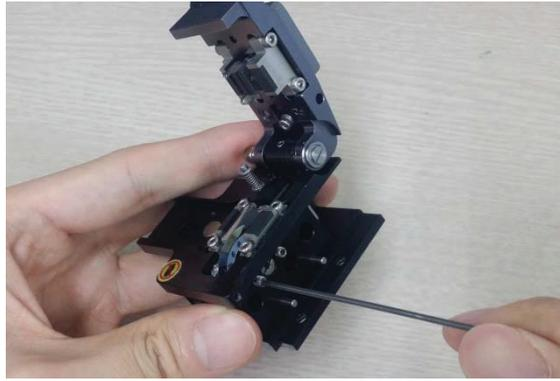
When the blade is adjusted to the proper height, tighten the set screw of slide. The height adjustment of the blade is closely related to cleaving quality . Make sure you perform height adjustment with BHS-01, sold separately. Please contact customer service for the information and availability of BHS-01.
